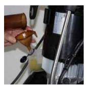
Pump oil tank with oil level sight and fill/empty function.
